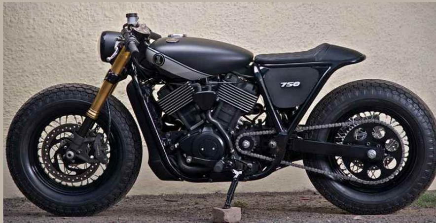
The exhaust note is basically a throaty growling sound with some popping. The 45° design of the engine thus creates a plug firing sequencing as such: The first cylinder fires, the second (rear) cylinder fires 315° later, then there is a 405° gap until the first cylinder fires again, giving the engine
